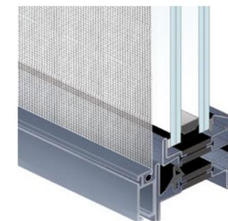
Fixed magnetized screens minimize the screen frame profile and allow for easy removal for convenient storage or cleaning.
