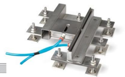
If concealment is your desired affect we have the perfect solution. A near seamless transition between floor coverings and stainless steel track is possible. The flush track's unique engineering provides adjustment screws allowing for a perfectly level installation. Included is a practical water drainage system.
